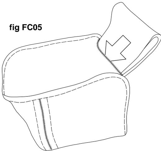
Push the other, narrower end of the foam stiffener down into the pocket running down the shorter side (FC05).
