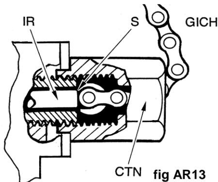
**3-speed.** Engage top gear, then move the control trigger to the middle position: the step, S, towards the end of the indicator rod, IR, should be level with the end of the axle, visible through the hole in the CTN. Next, select bottom gear, then middle, then top, and check that all three are engaging correctly.
