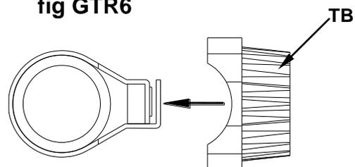
Next undo the clip screw CS and remove the trigger, leaving the metal clip on the handlebar. Re-use the old clip when fitting the new control unless it is damaged.
