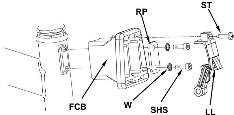
**The screw 'ST' must be fully screwed home:**
