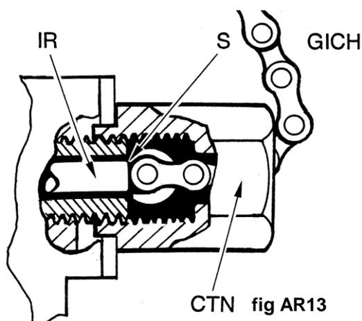
**3-speed.** Engage top gear, then move the control trigger to the middle position: the step, S, towards the end of the indicator rod, IR, should be level with the end of the axle, visible through the hole in the CTN. Next, select bottom gear, then middle, then top, and check that all three are engaging correctly.
