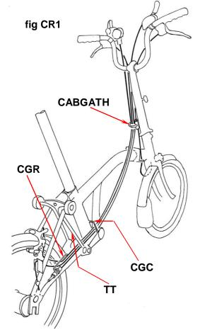
Let the other cables fall back down to their normal routing. Leave the forward end of the derailleur cable unconnected for the time being.
